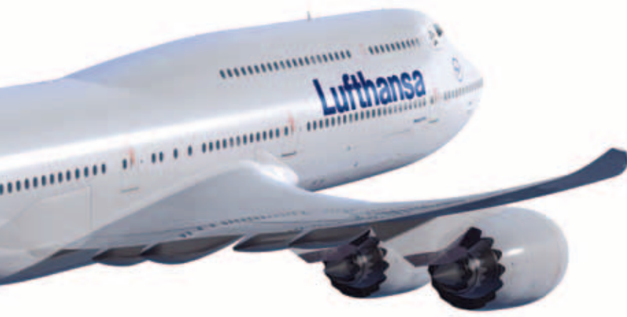
The chevron-shaped nozzle trailing edges on the Boeing 747-8 Intercontinental's GEnx-2B67 engines produce a significant reduction of jet noise.
