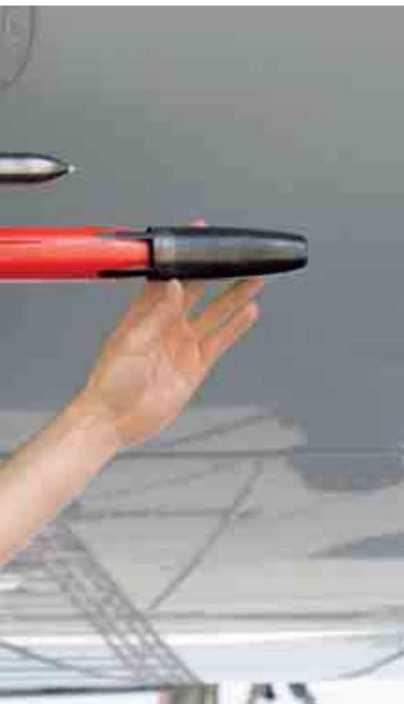
The air inlet system under the fuselage of the Airbus A340-600 christened "Leverkusen" collects climate data on long-haul flights at an altitude of 12,000 meters. Here, a Lufthansa Technik employee gives the adjustment a final check.
