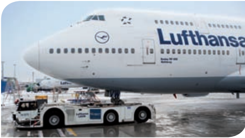
Comprehensive test run at Frankfurt Airport, using a Leos tow truck reconfigured as a TaxiBot test vehicle.
