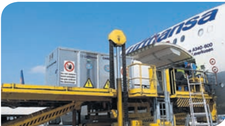
The CARIBIC measurement container is being loaded aboard the Lufthansa A340-600 "Leverkusen."
