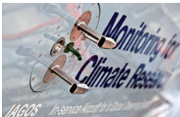
Project IAGOS: Measuring probe on the front left-hand fuselage of the Lufthansa Airbus A340-300 “Viersen.”
