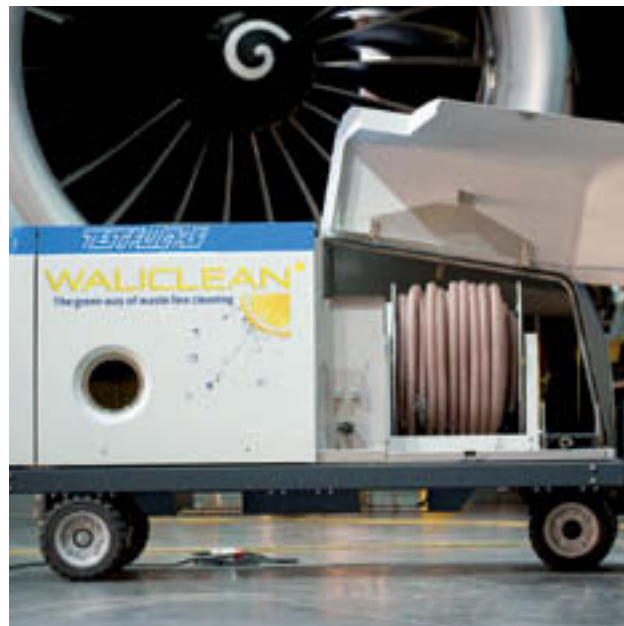
“Waliclean”: Technicians at Austrian Airlines developed this new cleaning system for low-pressure toilets.
