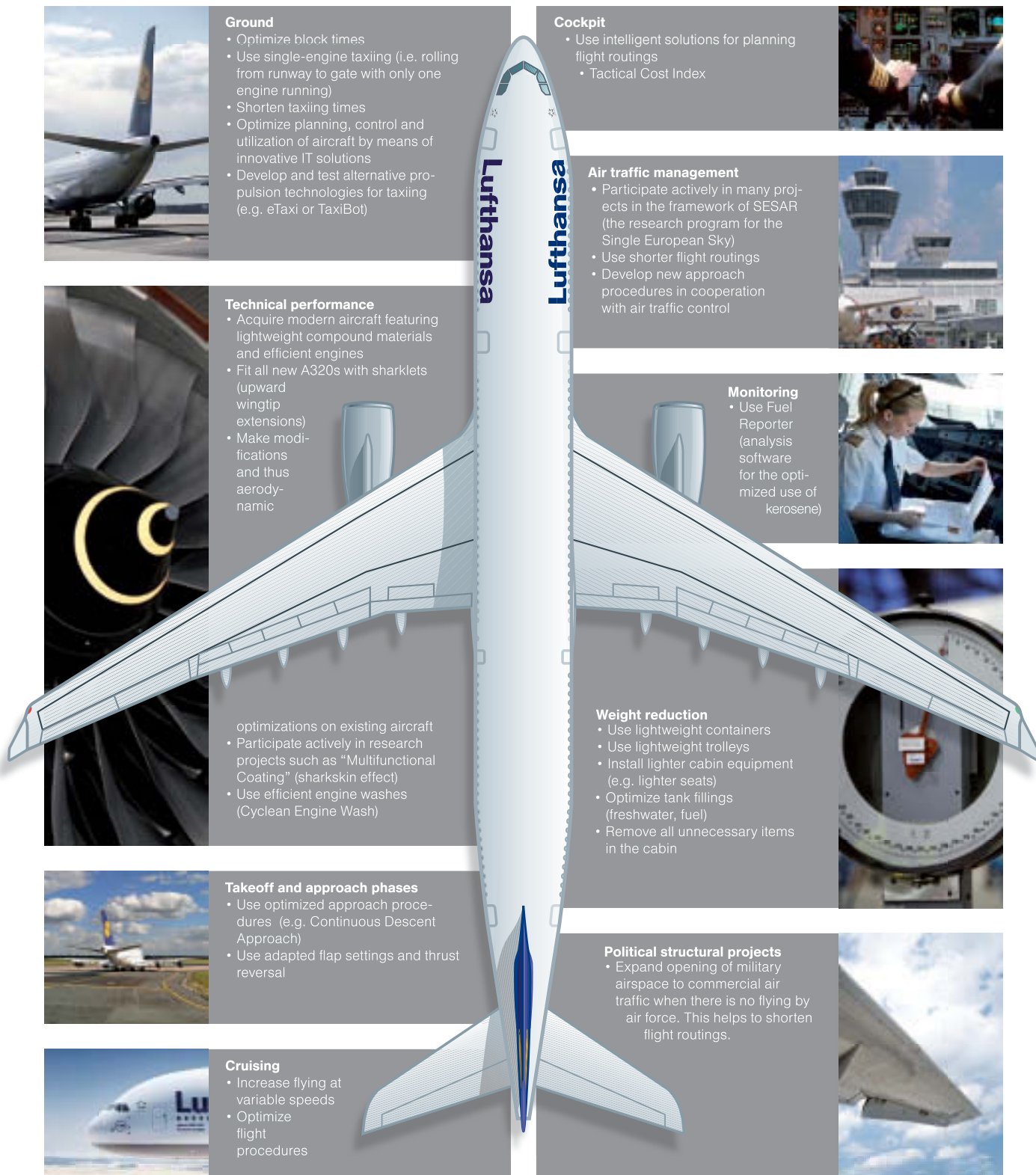
Measures to increase fuel efficiency within the Lufthansa Group (selection of examples)
