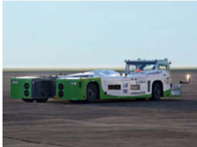
With TaxiBot, commercial aircraft can taxi to the runway with the engines off.
