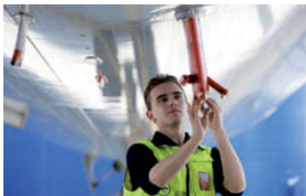
Project CARIBIC: Air intake system under the fuselage of the Lufthansa Airbus A340-600 “Leverkusen.”
