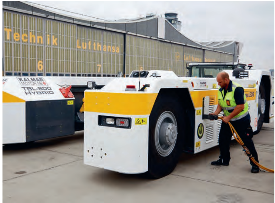
The eSchlepper diesel-electric hybrid aircraft tug is particularly suited for environmentally friendly maintenance and positioning tows of large passenger aircraft.
