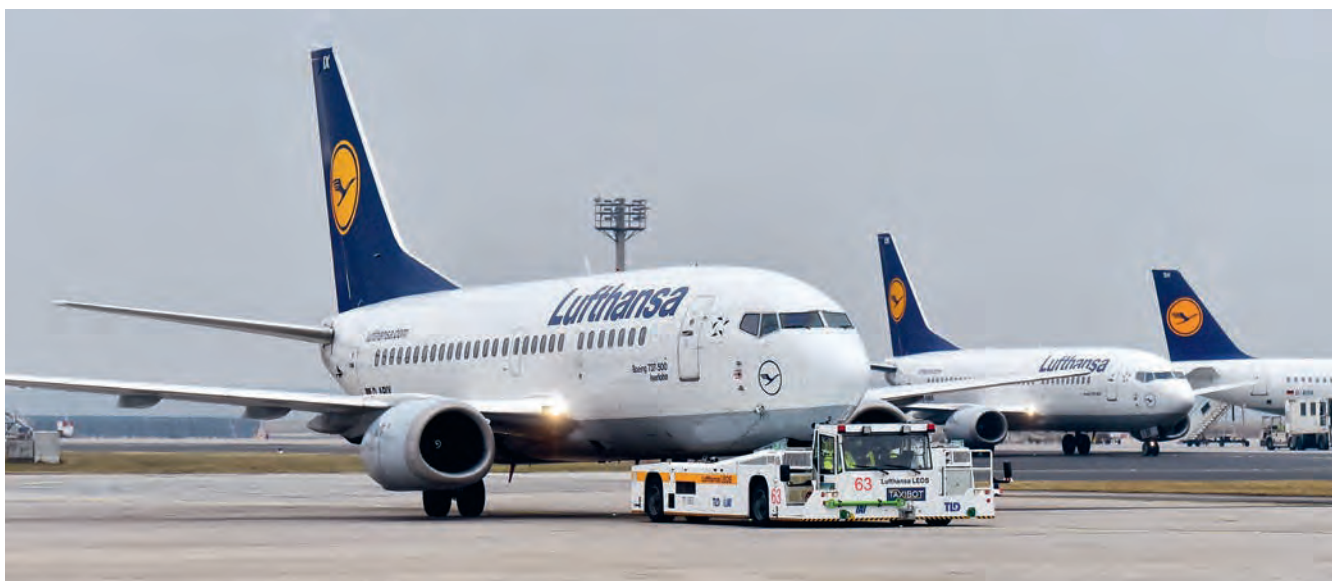
The TaxiBot hybrid aircraft tug allows pilots to tow the aircraft to the runway under their own command by using the Pilot Control Mode.
