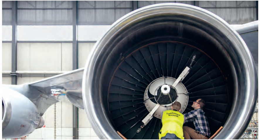
Cyclean®, the water-based engine wash developed by Lufthansa Technik, saves airlines time, maintenance costs and above all fuel. The company is researching the use of alternative blasting materials, such as CO 2 dry ice pellets, to make engine cleanings possible in permafrost regions as well.
