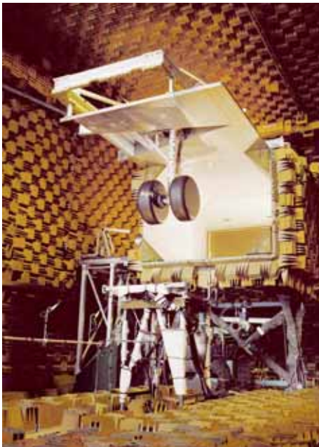
Wind tunnel trials aimed at determining the noise reduction potential on landing gears.
