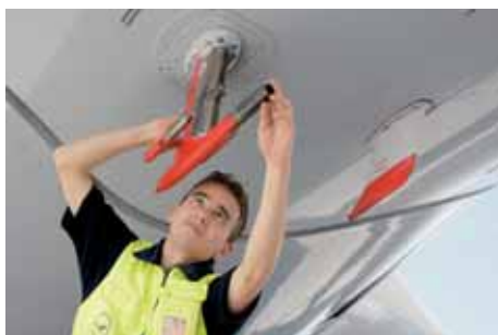
Commitment to climate research: The inlet system under the fuselage of the Lufthansa Airbus A340-600 "Leverkusen" collects climate data on long-haul flights at an altitude of 12,000 meters.
