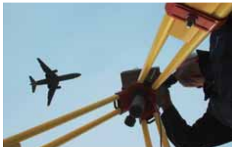
An acoustic camera allows scientists to pinpoint noise sources on an aircraft within a decimeter. Doing this also requires the accurate recording of the aircraft's position.
