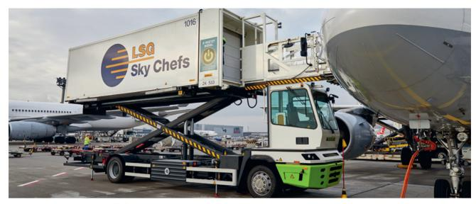
In the context of E-PORT AN, the LSG Group cooperated closely with external partners in the development of the fully electrified catering lift truck "eLift".
