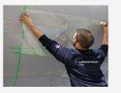
The film is being applied to the hull and nacelles first. Lufthansa Technik's engineers are already working on the ability to cover the wings with AeroSHARK film soon so that even more fuel can be saved and carbon emissions reduced.
