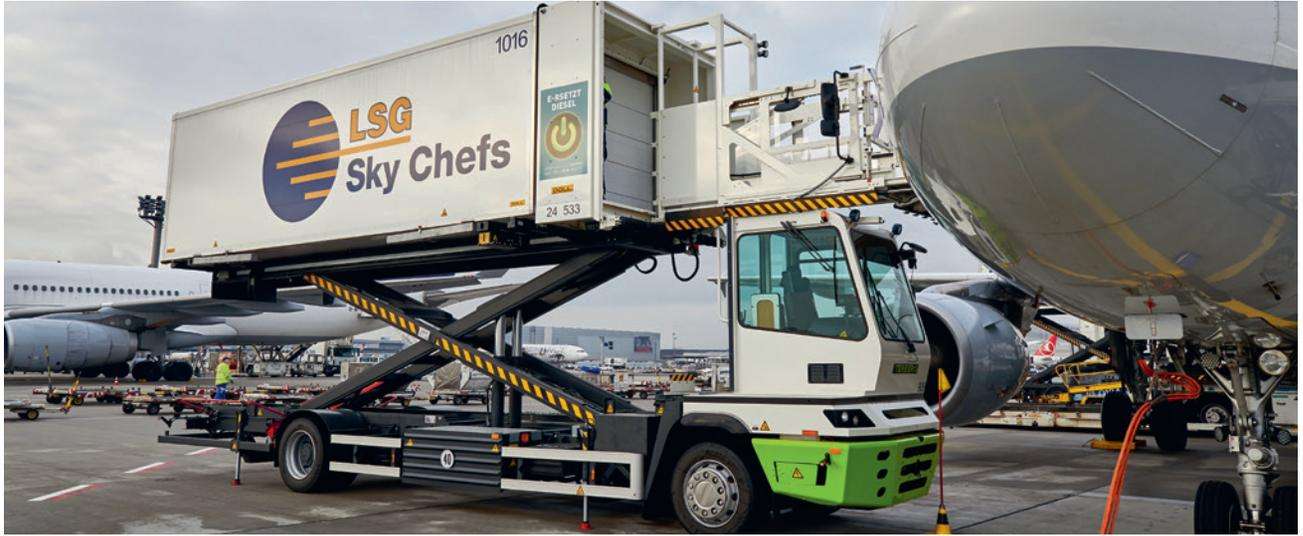
In the context of E-PORT AN, the LSG Group cooperated closely with external partners in the development of the fully electrified catering lift truck “eLift”.
